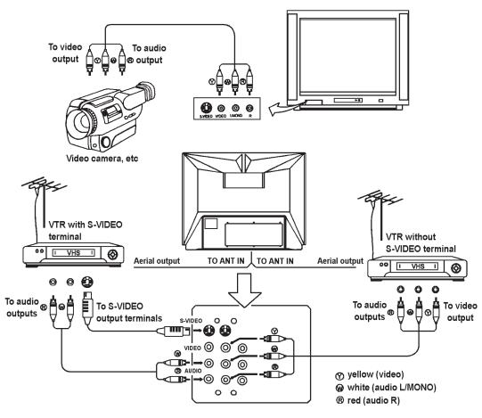
To select the input press the VIDEO button on the TV set or the AV button on the remote controller repeatedly until you see the corresponding input indication on the screen. To return to aerial input, press the AV button until it displays programme number, or press direct channel select button or the  $CH \blacktriangle / \checkmark$  button.
